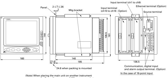
(Note) When placing the main unit on another instrument or on the floor, allow a space of 100mm or more between the unit and instrument or the floor.
